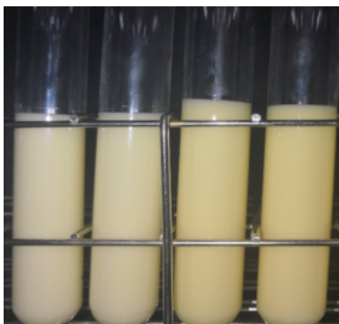
<Figure 3> Mayonnaises prepared using SD (spray-dried), FD (freeze-dried), SDE (spray-drying-enriched), and FDE (freeze-drying-enriched egg yolk powders) egg yolk powders
